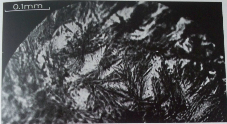
Fig. 3. — Photograph of Fern-like Crystals of PBN in Rubber
