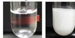
**Figure 3.**  $H_2$  LC (20 wt % water) and W/ $H_2$  emulsion (88 wt % water).
